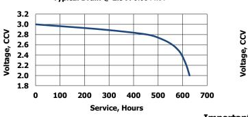
Load: 45K ohms - Continuous Typical Drain @ 2.9V: 0.064 mA Classification: Chemical System: Designation: Nominal Voltage: Typical Capacity:
